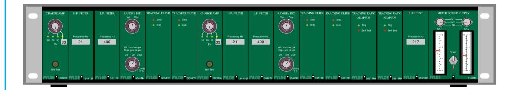
System depicted features 2 Differential Charge amplifiers for 2 channels and will give outputs of velocity and displacement. Twin meters allow immediate inspection of signals. All modules are plug in for instant upgrade or configuration change. Inputs are to the rear panel. Power is 115 or 230VAC 50/60Hz.
