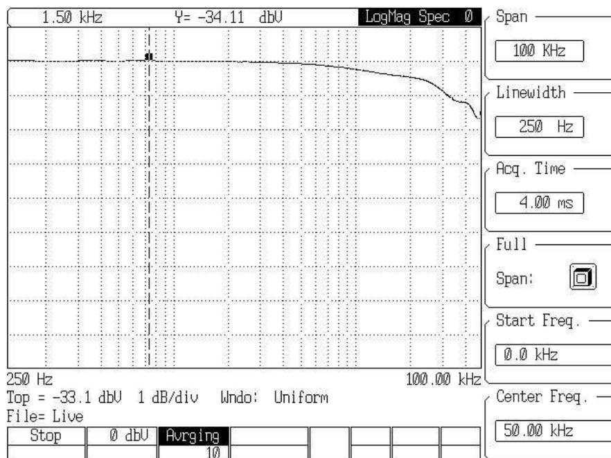
The above LP plot has a -3 dB cut off at > 100 kHz and is for LP filter by-passed and x100, x300 gain
