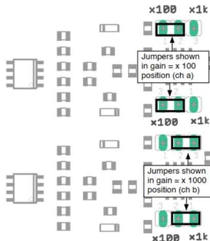
*Jumper positions for setting x 100 and x 1000 input gain*
