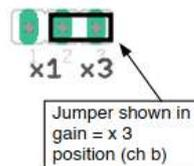
*Jumper positions for output gain of x 1 and x 3*
