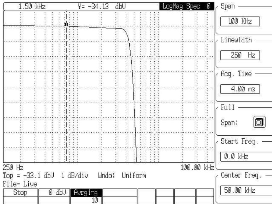
The above LP plot has a -3 dB cut off at 500 Hz and is for a 4k7 resistor pack
