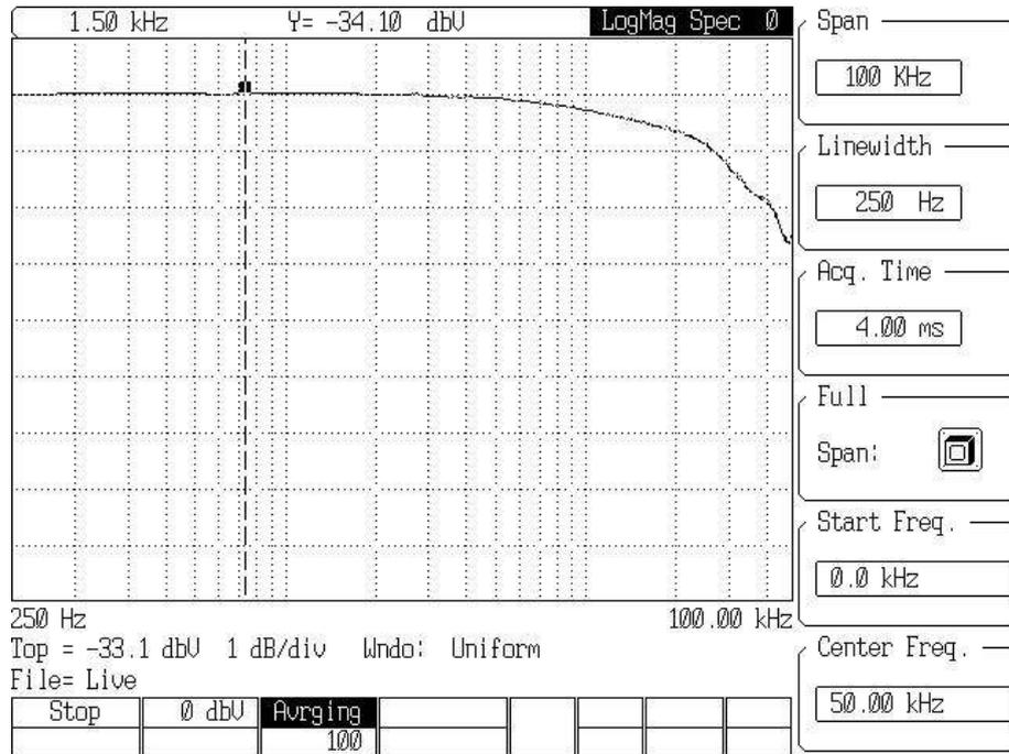
The above LP plot has a -3 dB cut off at > 100 kHz and is for LP filter by-passed and x1000, x3000 gain
