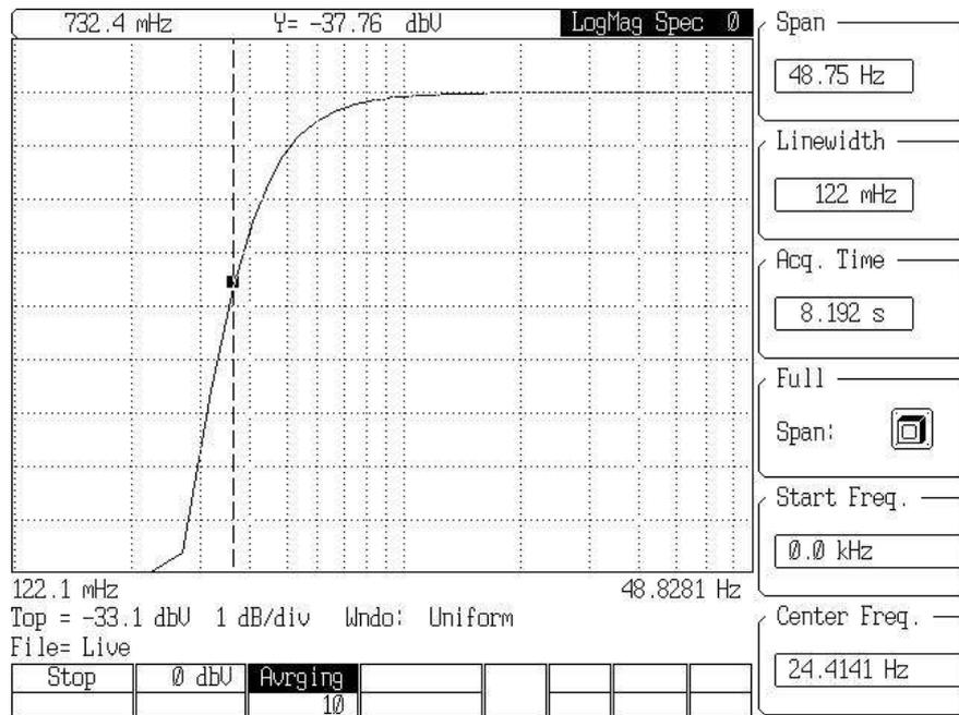
The above HP plot has a -3 dB cut off at 0.75 Hz and is for a 470 kΩ resistor pack
